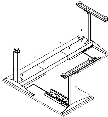
**Step 14:** Turn table right side up, adjust the glides as necessary, and plug the power cord into a 110v outlet.
