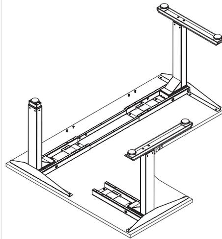
**Step 9 & 10:** Ensure the leg assembly is still centered, both side-to-side and front-to-back. Secure the leg assembly to the worksurface with **N** (12) truss head screws M5\*20mm. Secure the side bracket to the worksurface with **N** 12 truss head screws M5\*20mm.
