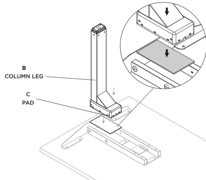
**Step 4:** Use 4 socket button head bolts, M6\*12mm to secure side bracket, column leg and crossbeam together as shown in detail.
