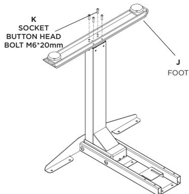
**Step 6a:** With option of Post foot: Attach O post foot to one column leg with K (4) socket button head bolts, M6\*20mm. Tighten bolts securely. Repeat step 6 with other two legs
