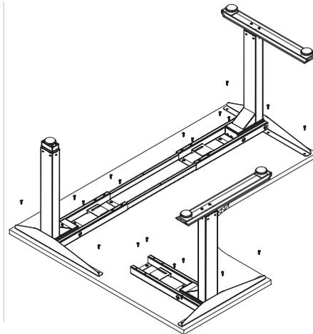
**Step 11:** Secure the **F** control panel in the desired location with **N** (2) truss head screws M5\*20mm. Insert the **G** control box in-between crossbeams.
