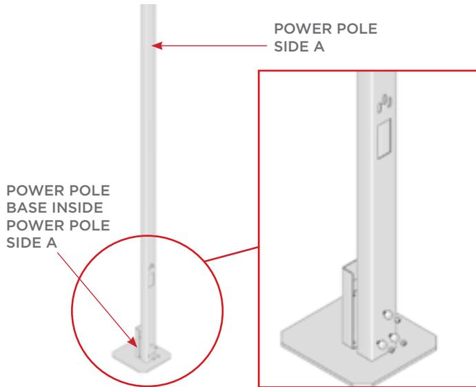
**STEP 5.** Secure using (3) M6\*12 screws, and (3) screw caps provided.
