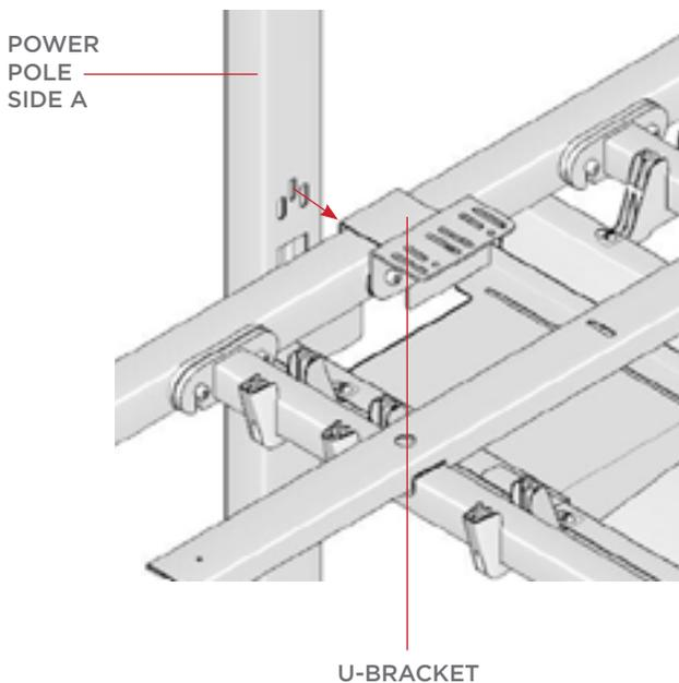
**STEP 6B.** Inside view of power pole side A mounted onto the U-bracket with (3) M6\*12 screws.
