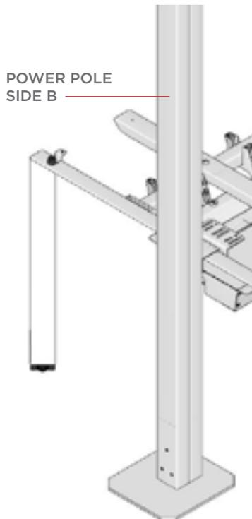
**STEP 10.** Finished assembly of the Double-Sided Power Pole.
