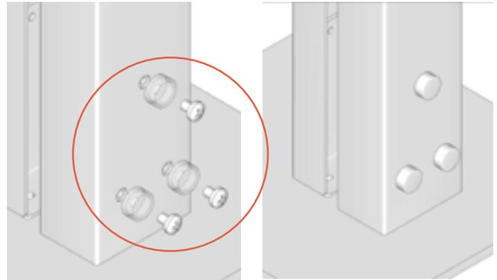
**STEP 6A.** Align power pole side A to the U-bracket. Secure using (3) M6\*12 screws provided.
