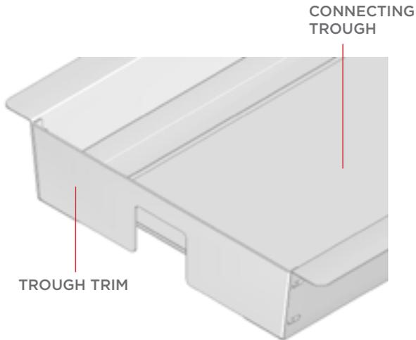
**STEP 8.** Secure trough trim using (4) self threading screws provided. Trough can now be installed into the Verity structure below the worksurface for Power Infeed to go through trough trim (Refer to Friant Verity Double-Sided manuals for Trough Installation)
