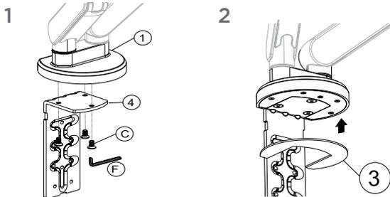
Use supplied allen wrench to attach to bottom support *clamp* with M6x 12mm screws (3).
