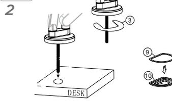
Attach monitor arm to desk, by inserting the base with the screw into the predrilled hole. Before you merge your monitor arm and your desk, make sure you are using the anti-slip rubber *grommet*.
