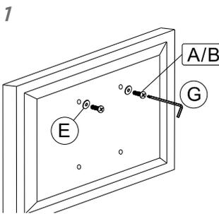
Using M4x 12 mm or M5x 12mm screws, screw into the top holes on the back of the monitor.
