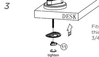
Attach anti-slip rubber *grommets* (2) to the pressure plate. Attach the pressure plate to the bottom of the worksurface by screwing everything together with the knob nut.
