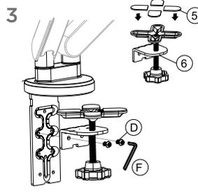
Using the allen wrench, attach the knob to the bottom support using M6x 10mm (2) screws. Place anti-slip rubber on top of the installed knob.
