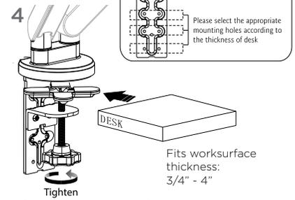
Insert desktop in the gap between the monitor arm and the bottom support. Place the cable cover over exposed cables.
