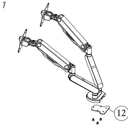
Attach the bottom support *verity* to the monitor arm with screws (3).
