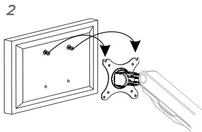
Position monitor by aligning screws with grooves in the upper corners of the monitor attachment bracket.
