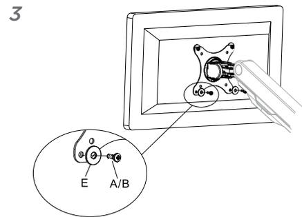
Using the bolts (2) and M4x 12mm (2) or M5x 12mm (2) to secure the monitor to the monitor arm.
