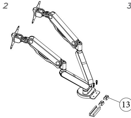
Insert the blocks (2) into the Verity track. Then, using screws, attach the monitor arm bottom support to the blocks (2).
