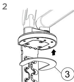
Attach anti-slip rubber *clamp* to the bottom of the monitor arm.
