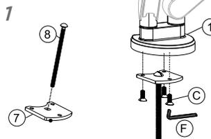
Insert screw into bottom support *grommet*. Use allen wrench to attach bottom support *grommet* to monitor arm by using M6x 16mm screws (3).
