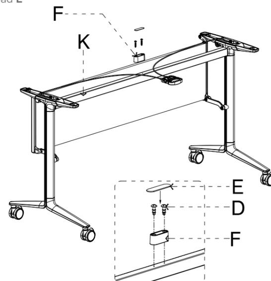
Step 2: Attach fixed support bar K to base kit N using (2) bar supports H
