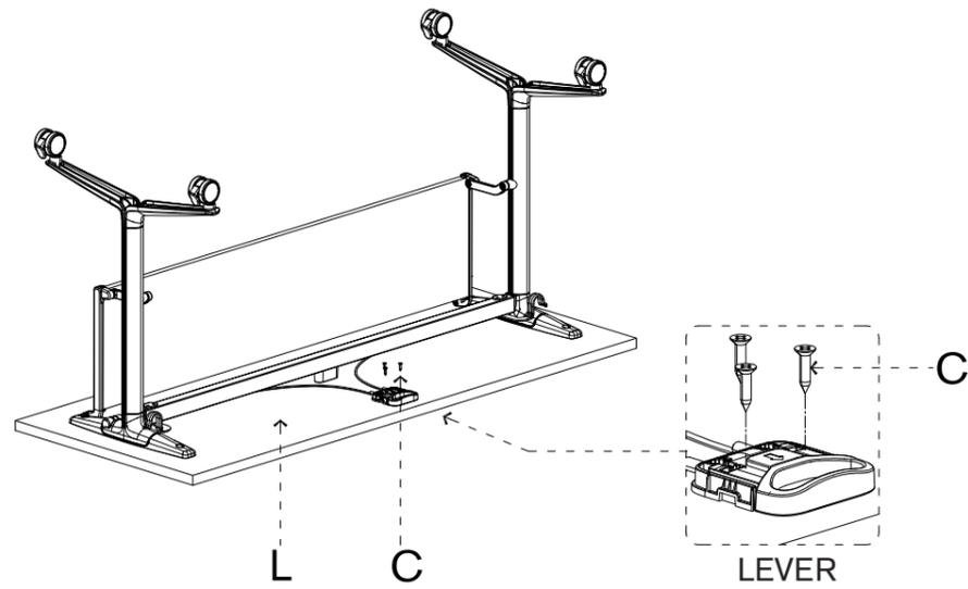
**Step 9:** Fold the base kit N by pulling on the lever.
