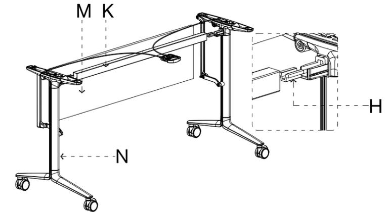
Step 4: Secure modesty panel M to base kit N using (4) wood screws C
