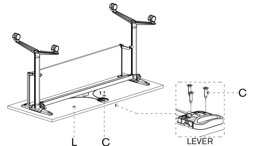
**Step 8:** Fold the base kit N by pulling on the lever.
