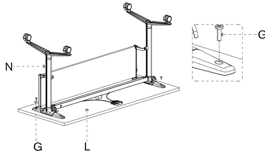
Step 7: Secure the lever to the work top L with (3) wood screws C
