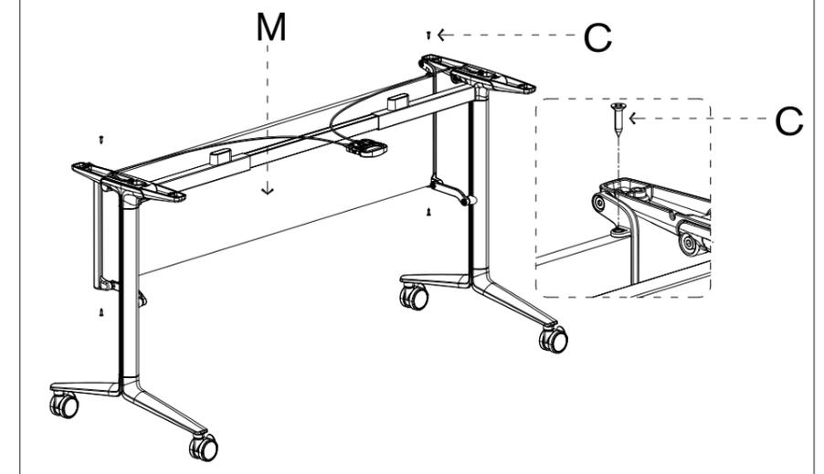
Step 5: Flip the base onto the backside of the worktop L as shown in image
